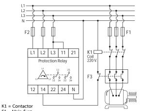
F1 = Main fuse F2 = 2 Amp fast acting fuses recommended for safety (Not required)
